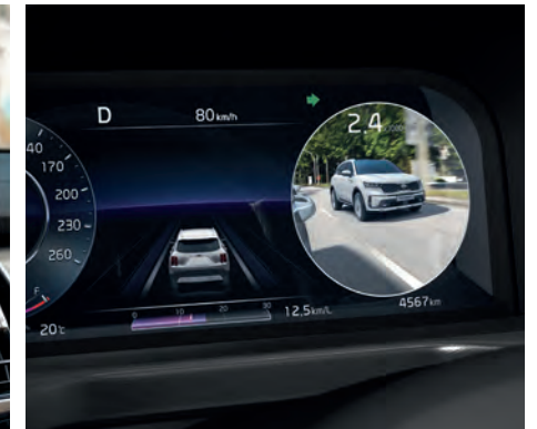
BLIND-SPOT MONITOR 1,2 activates within the instrument panel when you turn on the blinker to change lanes, to display the blind spot in the direction of your turn signal
